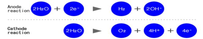
Raw water containing calcium ions is put into the electrolysis tank. When a direct voltage is applied, direct current flows and the positive ions (M +) such as calcium ions, magnesium ions, potassium ions, sodium ions, etc. are attracted to the anode
